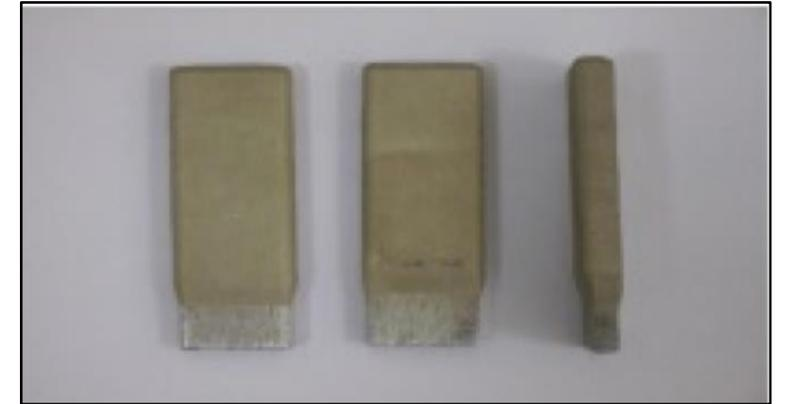
Lastrine in acciaio AISI 304 con coating Cold Spray Ni – Al 50% -50%, 90%-10% e 95%-5%
